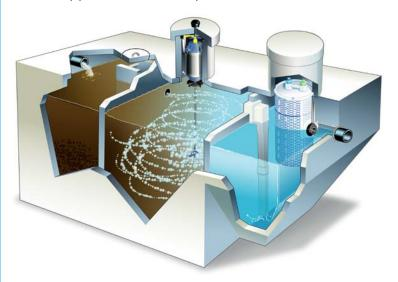
Seamlessly integrating several proven technologies, the Singulair® Direct Bury UV NPDES system's primary treatment platform is the Model 960 equipped with Service Pro® remote monitoring. The UL Listed Service Pro® control center automatically notifies service providers if a component alarm is detected.
